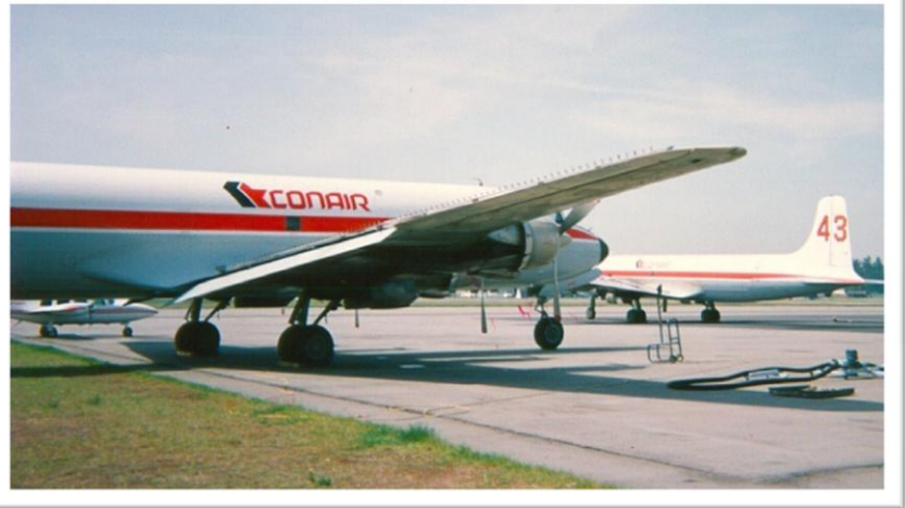
Figure 44: Spray converted Conair DC6's based out of the Abbotsford Tanker Base
