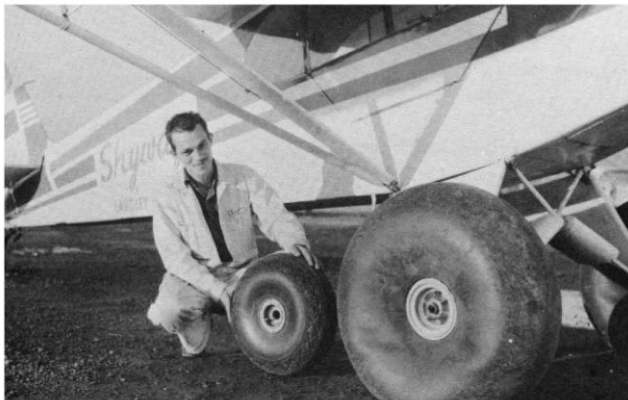
Figure 18: A Skyway Air Services Super Cub - illustrating oversized tires for use in soft, rough field operations
