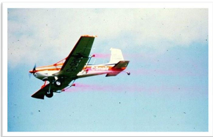
Figure 24: Conair Agwagon - spray calibration with Rhodamine dye
